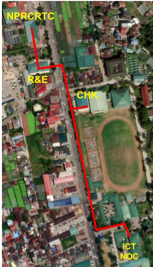
Figure 0. Outdoor Fiber-optic Network Layout
